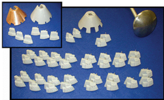
Fig. 5 Aftbody pieces for the Apollo-era (inset) and Orion-derived model shapes including various RCS jet configurations.
